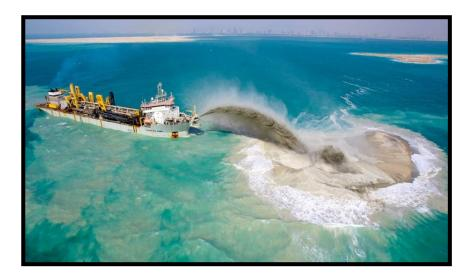
Figure 4: The process of rainbowing sand to create Palm Jumeriah's fronds
