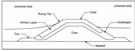
Figure 4.0: Typical Rubber-Mound Cross Section Source: http://www.ipenz.org.nz/ipenz/publications/transactions/transactions98/civil/4palmer.pdf
