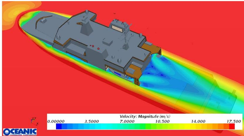
**Figure 7.** Velocity distribution of airflow past a vessel
