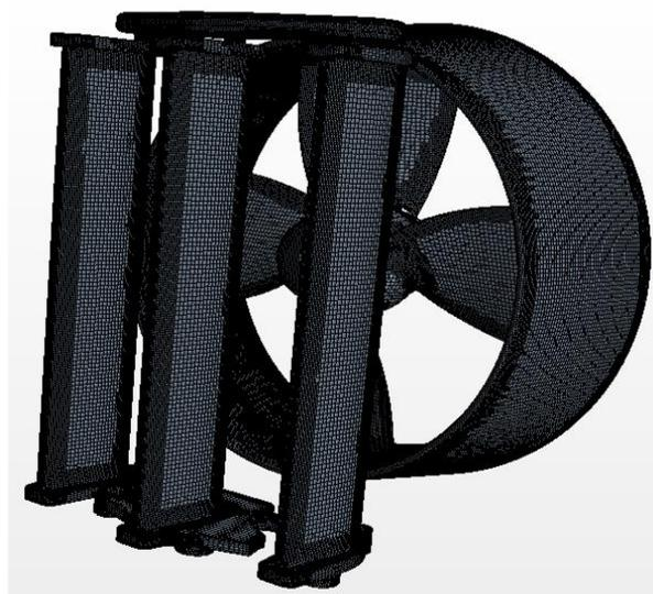
**Figure 5.** Study of propeller-nozzle-rudder interaction
