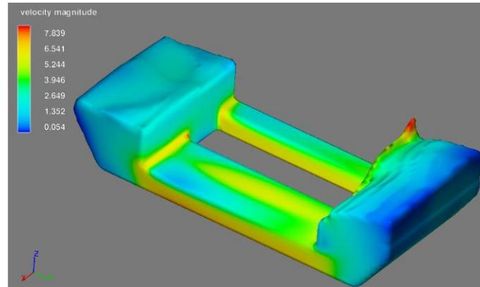
**Figure 11.** Velocity magnitude contour from U-tube tank simulation
