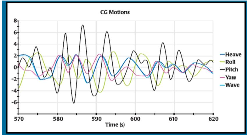
Figure 13. Time history of ship CG motion from MOTSIM simulation
