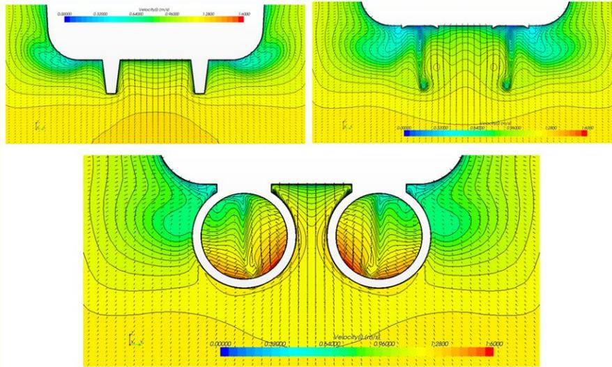
Figure 3. Flow study of articulated tug barge (ATB) – cross sections
