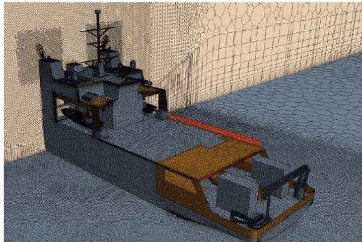
**Figure 8.** Meshes of airflow pass a vessel
