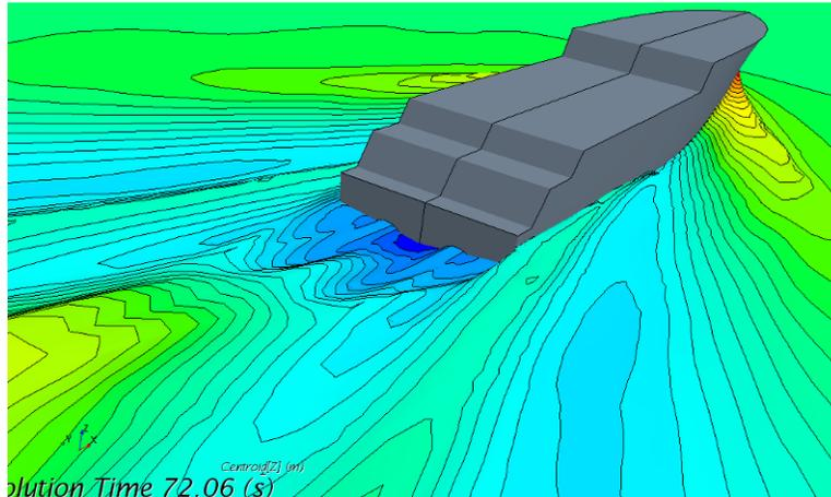
**Figure 1.** Flow study of high speed vessel
