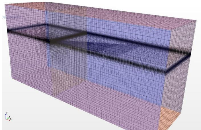
**Figure 2.** Mesh for high speed vessel, showing fine grid at water air interface
