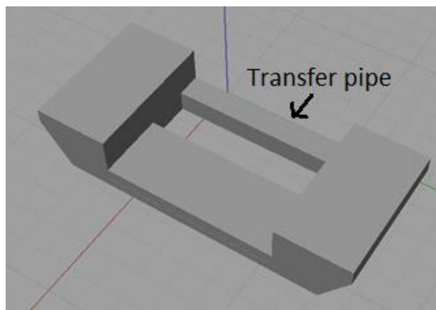
**Figure 9.** Geometry of a U-tube tank
