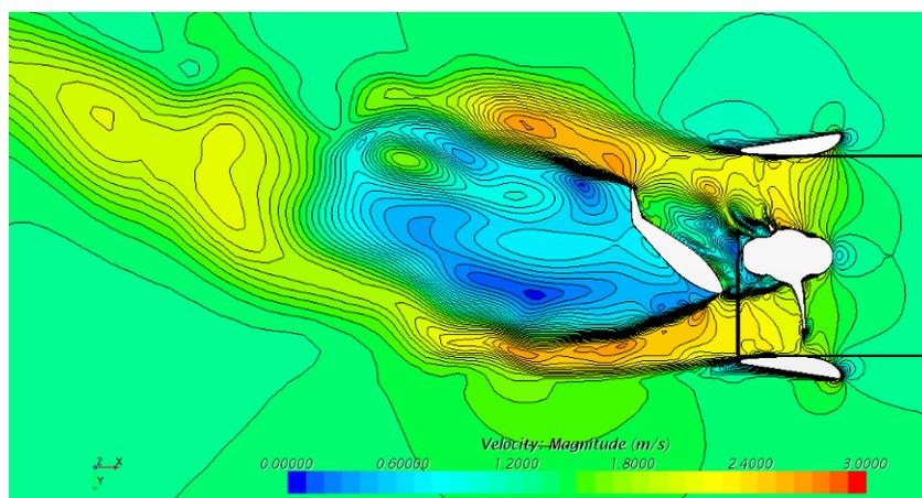
**Figure 6.** Velocity distribution of propeller-nozzle-rudder interaction
