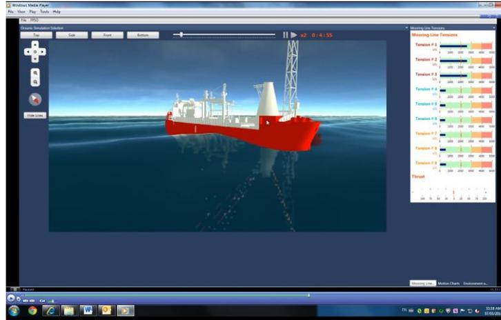
Figure 15. Screen shot of FPSO motion visualization
