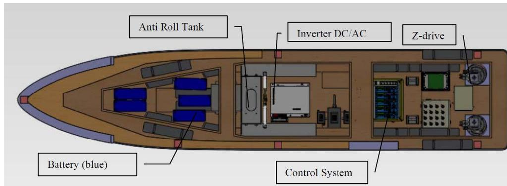
**Figure 10.** U-tube tank position in a vessel
