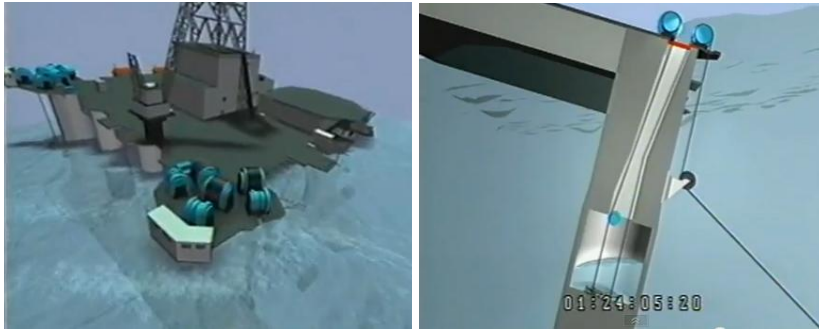
Figure 5: Simulated illustration of the forward list (left) and chain lockers filling with water (right) [6]
