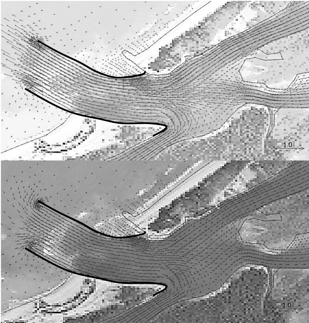
Figure 4 Entrance flow paths during ebbing and flooding tide
