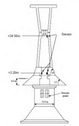
Figure 6: Typical Cross section of pier with tilt-meter locations. Figure retrieved from [2].
