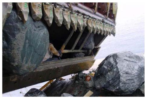
Figure 6: Boulders being cleared from Vasco da Gama's draghead [7]
