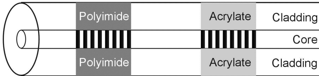
Figure 1. Illustration of fiber Bragg gratings coated with different polymers for sensing.
