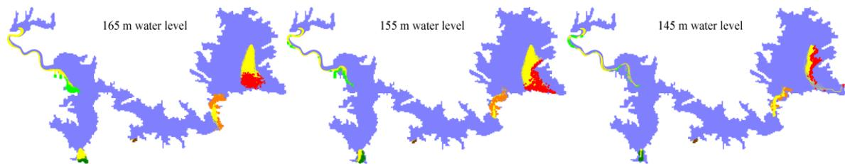
Figure 4. Oil spill trajectories at three initial water levels (the yellow color is the oil spill trajectories, and the other colors at the end of the oil trajectories are the locations of the oil parcels after 15 days, from different potential oil spill sites)
