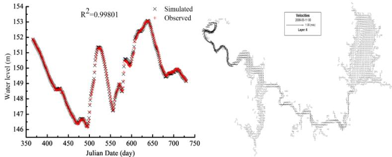
Figure 2. The time series of simulated water levels (cross) and the observed data (plus) at the Danjiangkou Dam area, and the simulated flow direction on May 11, 2009
