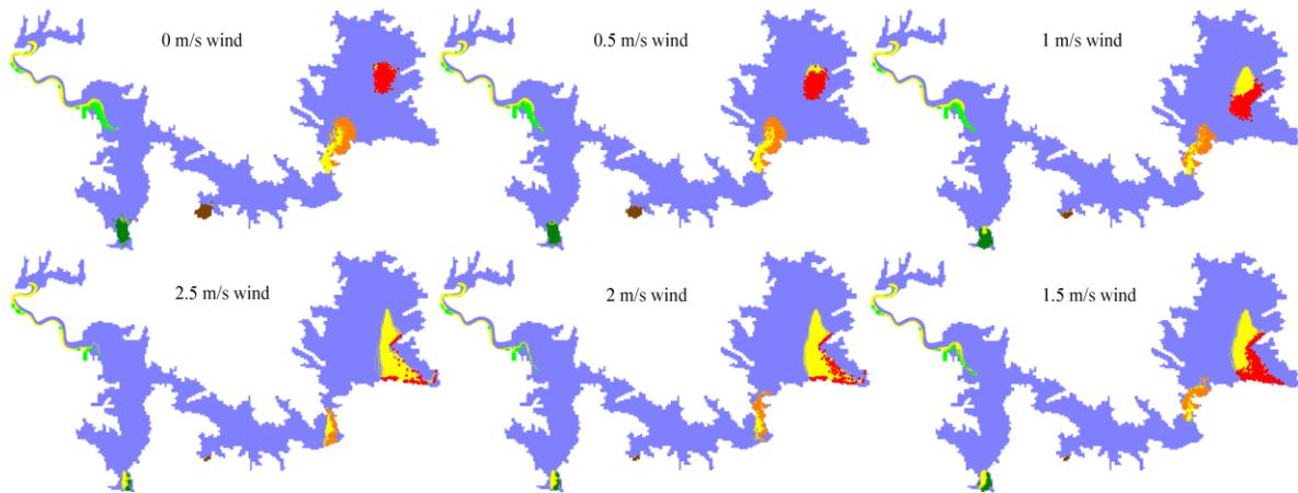
Figure 7. Oil spill trajectories during different wind speeds (the yellow color is the oil spill trajectories, and the other colors at the end of the oil trajectories are the locations of the oil parcels after 15 days, from different potential oil spill sites)
