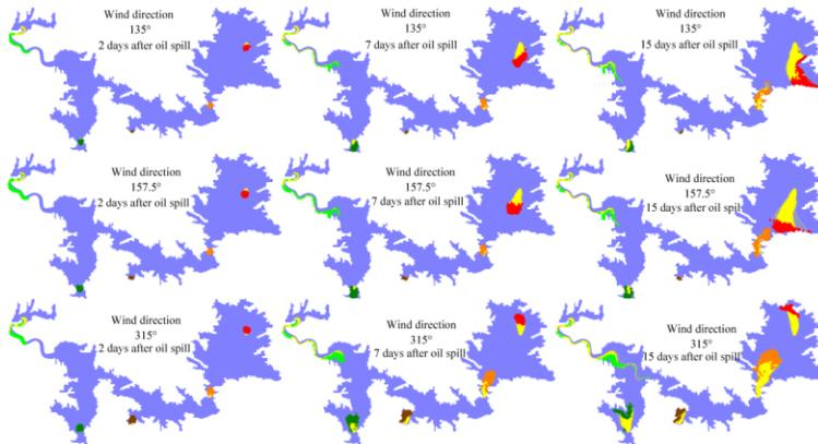
Figure 8. Temporal and spatial patterns of oil parcels during the top three most frequent wind directions (the yellow color was the oil spill trajectories, and the other colors at ends of the oil trajectories are the locations of the oil parcels after 15 days, from different potential oil spill sites)
