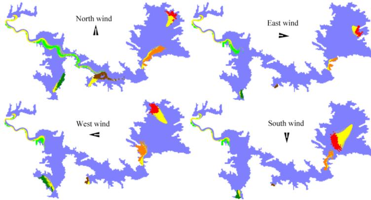
Figure 6. Oil spill trajectories for different wind directions (the yellow color is the oil spill trajectories, and the other colors at end of the oil trajectories are the locations of the oil parcels after 15 days, from different potential oil spill sites)
