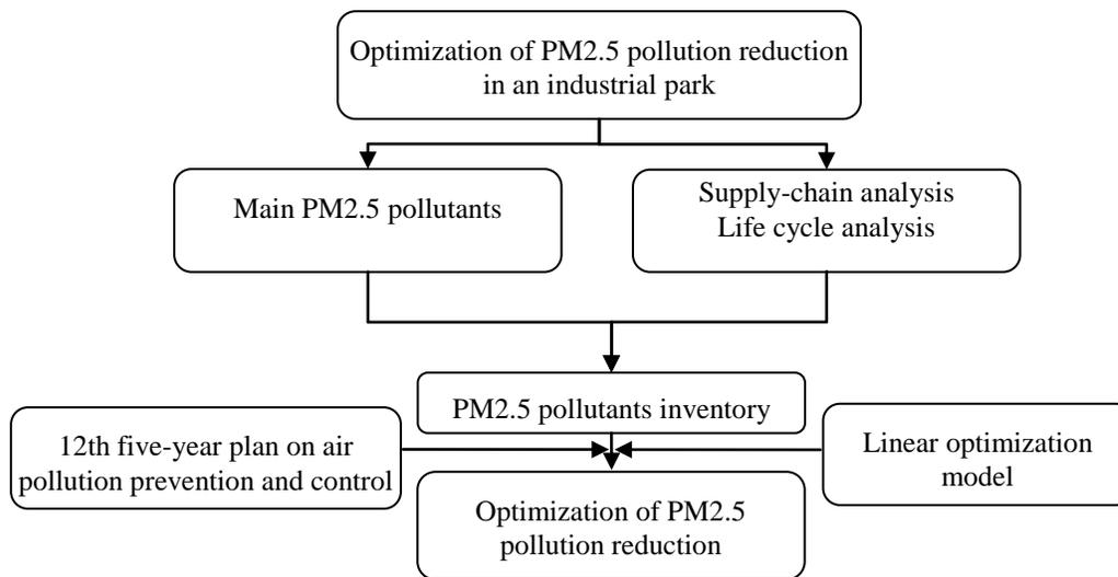
**Fig. 1** Optimization system for PM2.5 emission reduction in an industrial park
