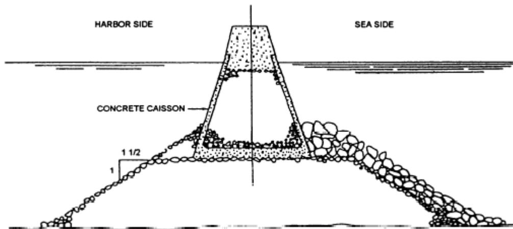
Figure 2: Sample detail of a composite breakwater
