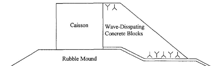
Figure 3: Geometry of wave dissipating concrete blocks against composite breakwaters
