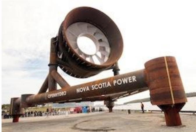
Figure 5: Nova Scotia Power and OpenHydro In-Stream Tidal Turbine [9]
