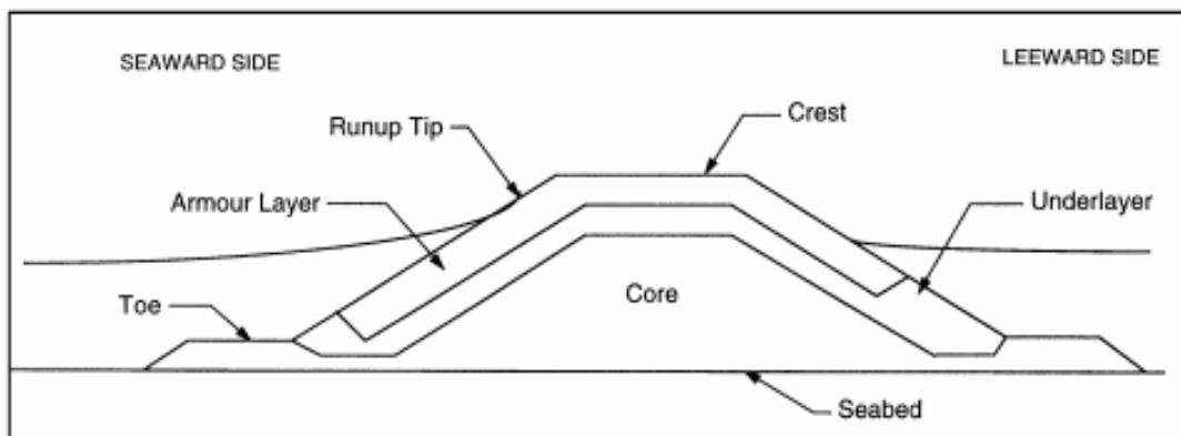
Figure 4.0: Typical Rubber-Mound Cross Section
