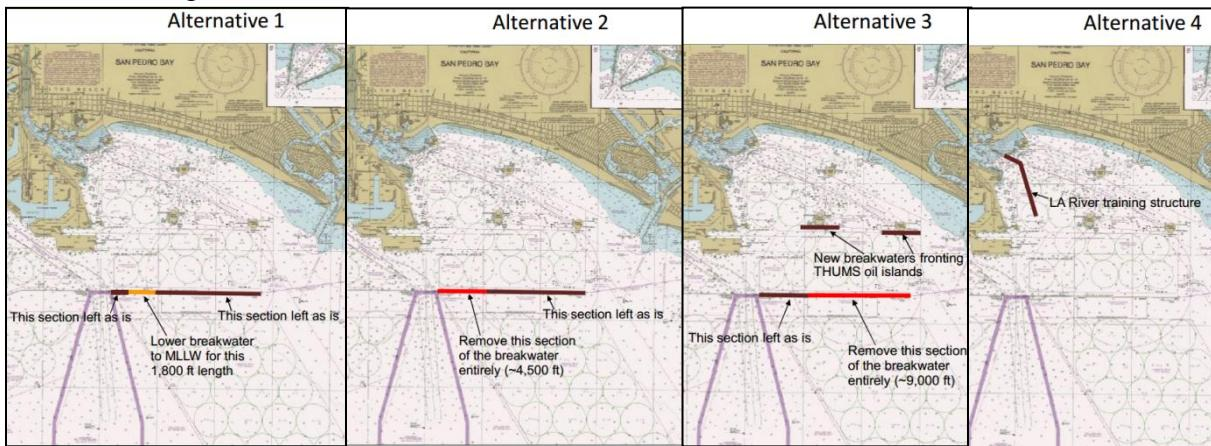
**Figure 6.0: Alternate Breakwater Designs**
