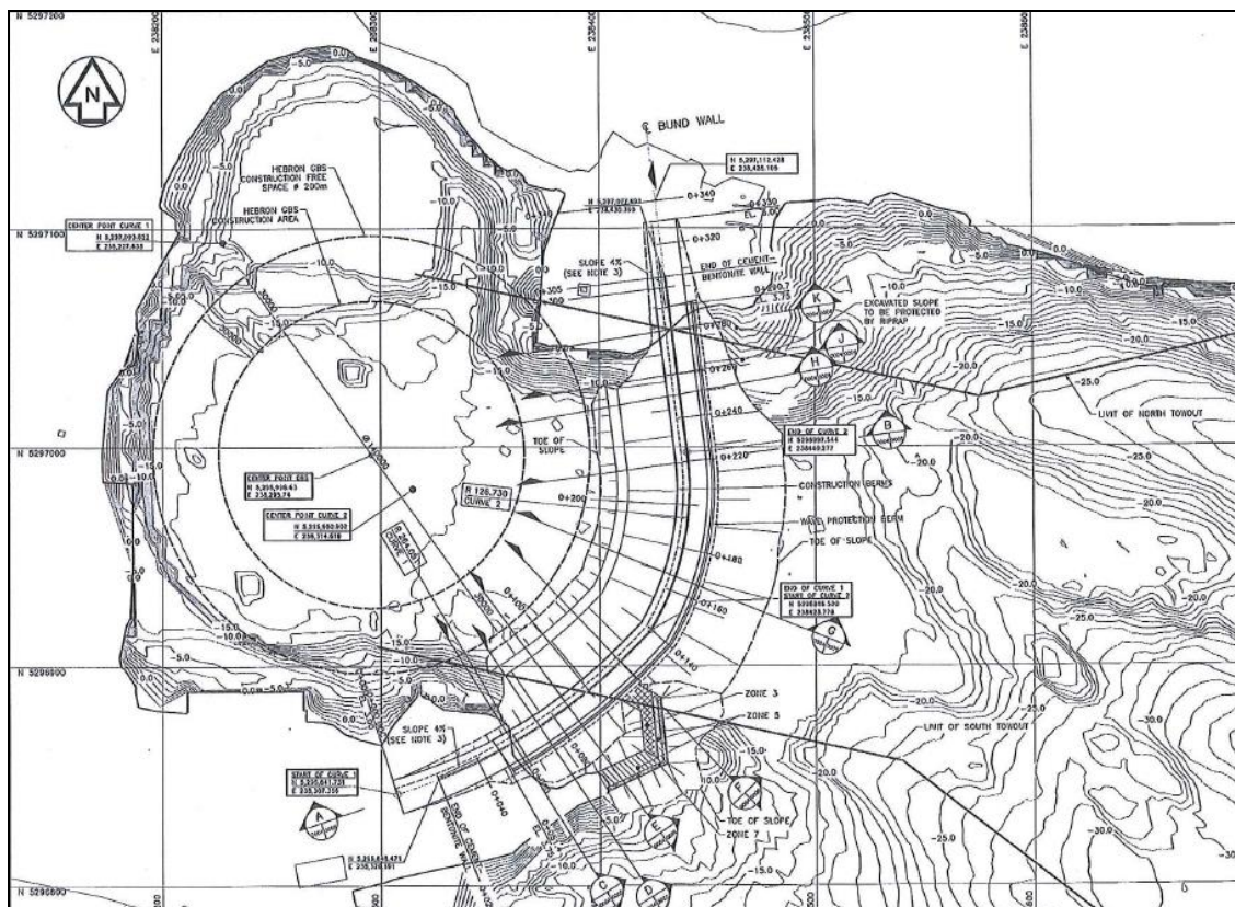
Figure 7 – Detailed Bull Arm Drydock Bathymetry and Hebron Bund Wall
