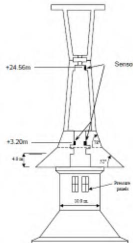
Figure 6: Typical Cross section of pier with tilt-meter locations. Figure retrieved from [2].
