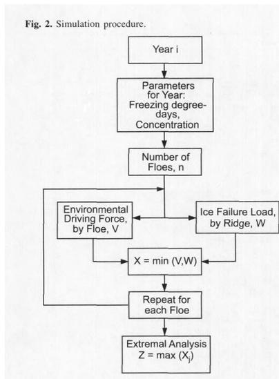
Figure 4: Simulation Procedure. Figure retrieved from [2].
