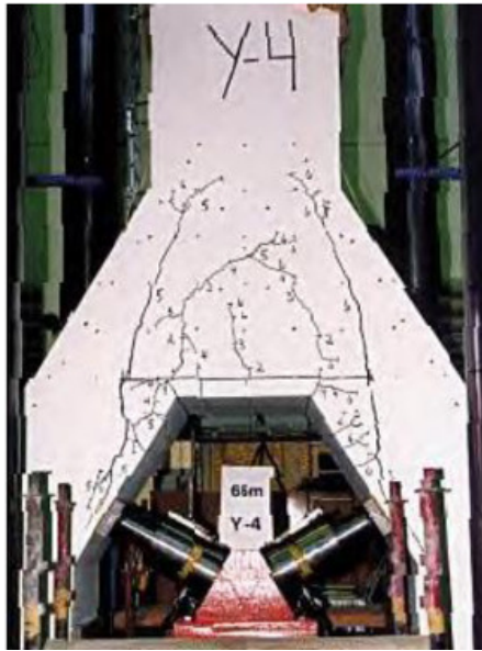
Figure 4 - Experiment test of a tricell joint [4]
