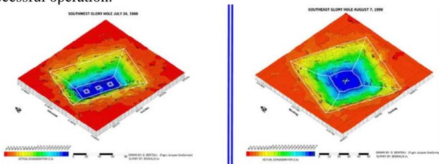
Figure 5: Drill Centre profiles as completed by the *Queen of the Netherlands*, summer 1999 [7]
